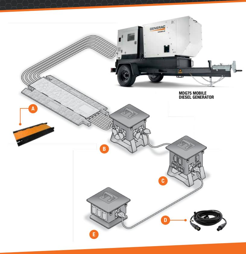
Spider boxes convert the power from the mobile generator to usable, accessible receptacles for a variety of jobsite power needs.
