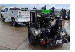
performance dry prime feature enhances efficiency and enables faster pump priming and set-up. All-in-all, this unit helps save time which translates to saving money."
